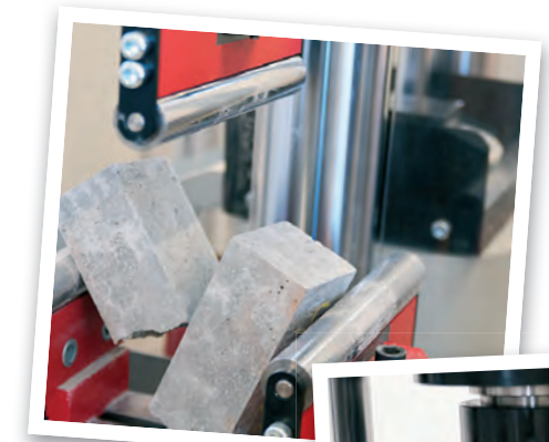
Determination of cold modulus of rupture. EN1402-6
