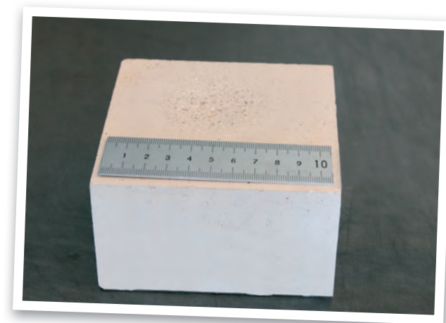
Testing the resistance to abrasion. ASTM 704C
